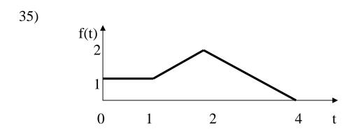
i-Write f(t) in terms of unit step function.ii-Find the Laplace transform of f(t).
